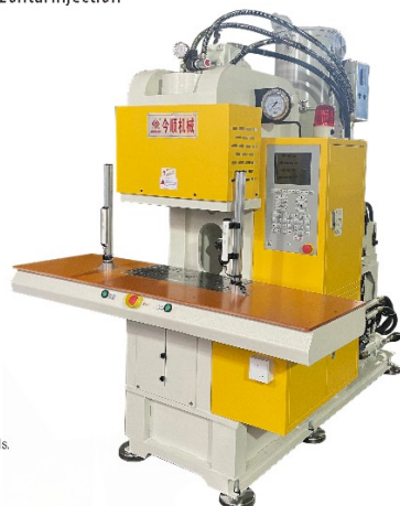
◆ 锁模力/Clamping Force: 55-85T ◆ 射出量/Injection Weight: 1g-278g JC-550T 伺服节能注塑机
